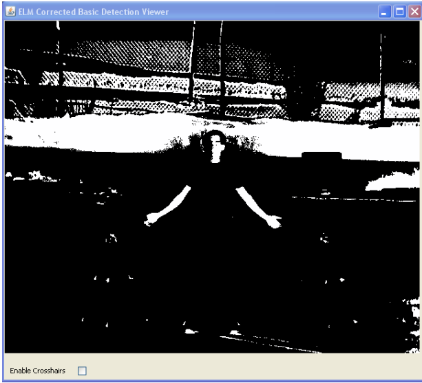
Figure 30. Output of the basic skin detection (NDSI only) algorithm and ELM. Notice the large number of snow pixels that are declared as skin.
