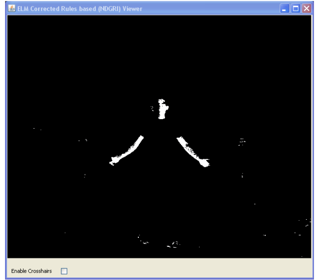
Figure 31. Output of the rules based (NDGRI and NDSI) Detection Algorithm and ELM. Notice that the snow is not declared as skin in this image.
