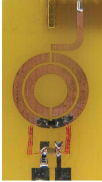
Figure 3.10: Variable-capacitor-diode mounted on an SRR device [82]
