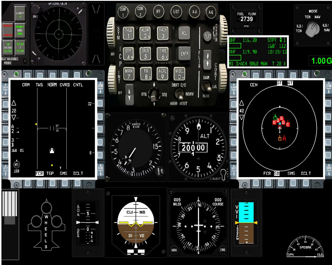
Figure B.8: Generic Heads Down Display
