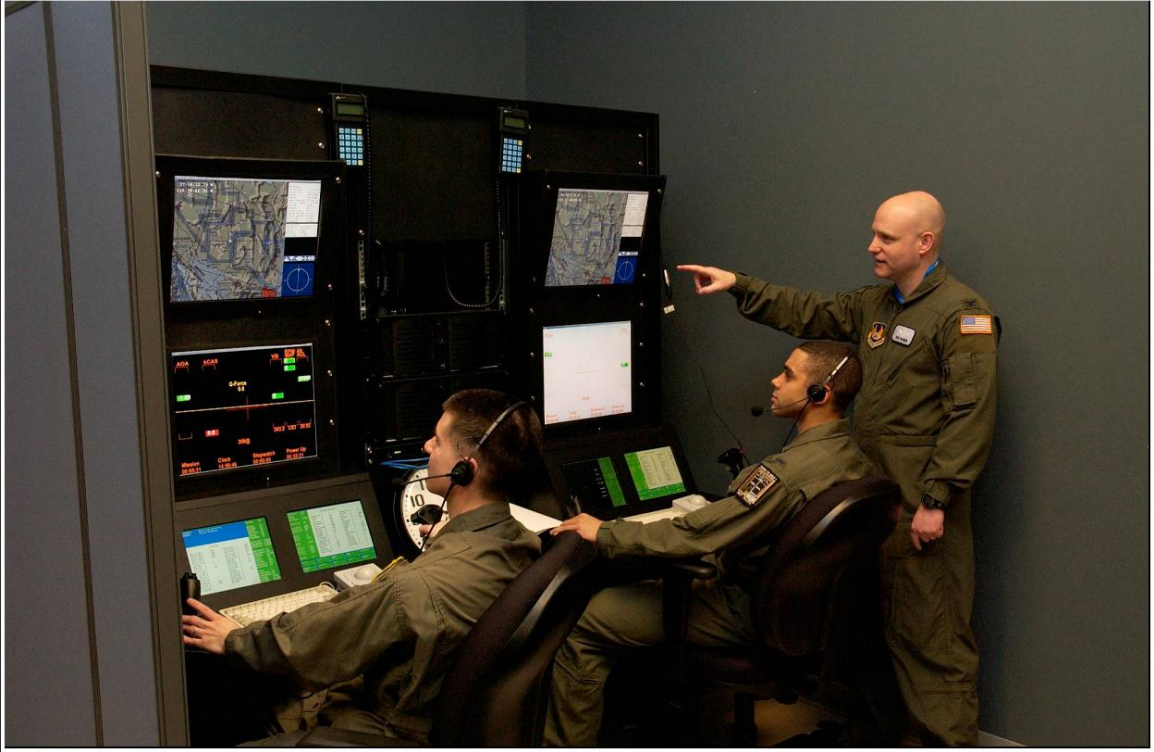
Figure B.9: MQ-9 Ground Control Station
