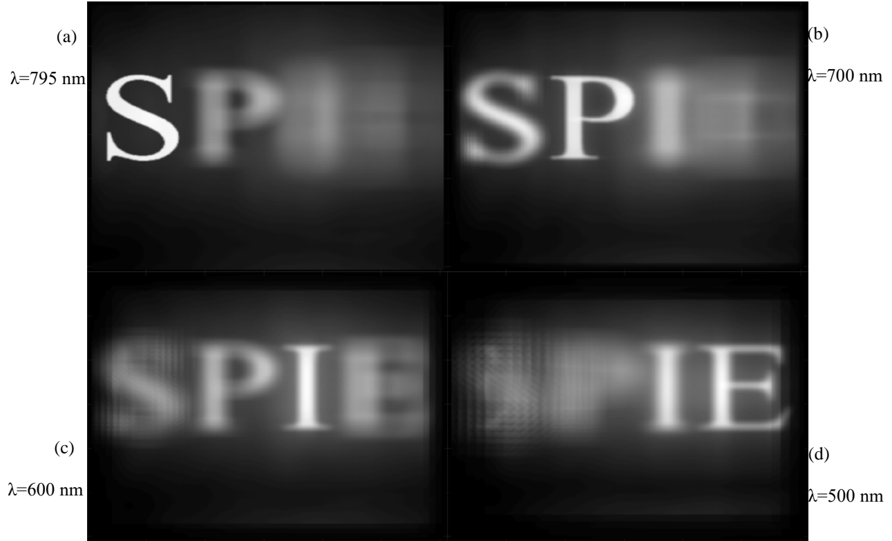
Figure 25. Hyperspectral image refocused with the Gaussian smoothing algorithm at a) 795 nm, b) 700 nm, c) 600 nm, and d) 500 nm. The image contrast was adjusted to keep the image brightness comparable between images. The Gaussian smoothing algorithm is able to refocus very well near design to differentiate wavelengths, however, as we get farther from design, that ability to differentiate wavelengths well disappears. This matches the results from DR.
