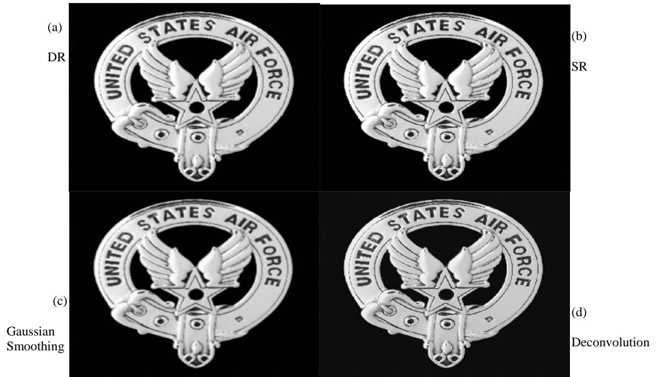
Figure 19. A more complicated image of an Air Force pin with various levels of brightness simulated to emit at 795 nm. Image is refocused using a) DR, b) SR, c) Gaussian smoothing, and d) deconvolution algorithms. All algorithms are able to accurately refocus the image near the design wavelength and since this is in the range of perfect refocusing, the algorithms all produce similar results.
