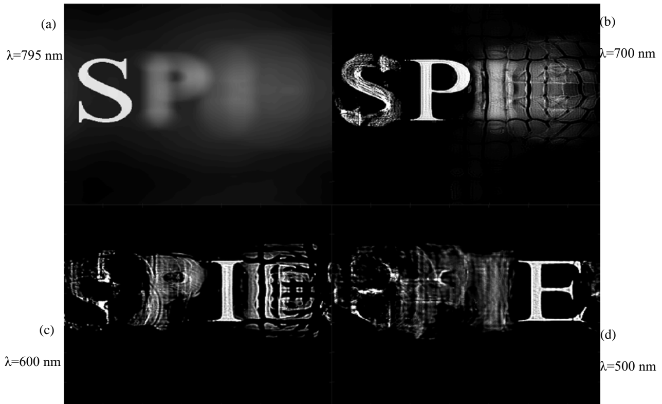
Figure 26. Hyperspectral image refocused with the Deconvolution algorithm at a) 795 nm, b) 700 nm, c) 600 nm, and d) 500 nm. The image contrast was adjusted to keep the image brightness comparable between images. The deconvolution algorithm is able to separate the wavelengths near design and far from design. It does not completely get rid of the images that are recorded at wavelengths other than the wavelength being refocused at, but the image is blurry enough to imply that the algorithm should be rerun at other wavelengths to test for alternate source wavelengths.
