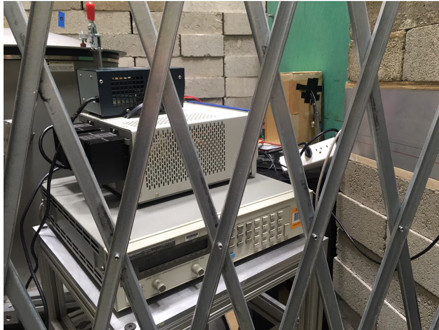
Figure 38. The setup used at Ohio State University. The thermal neutron port is perpendicular to the test Eu:LiCAF wafer, which is located in the box that is adjacent to the far wall. The three pieces of equipment on the cart are power supplies.
