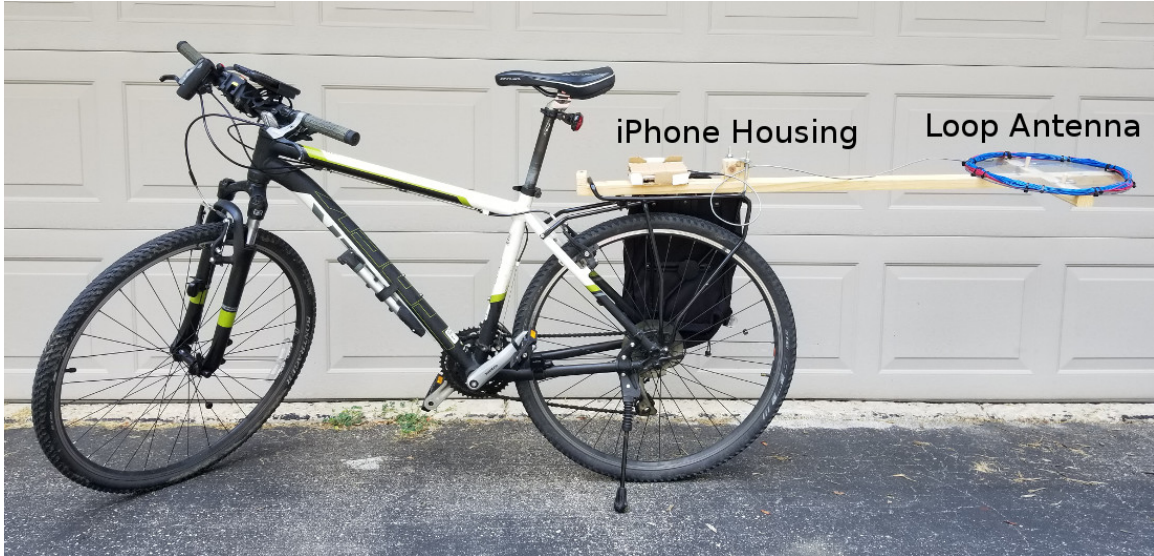
Figure 26: Bicycle with loop antenna attached to the back.
