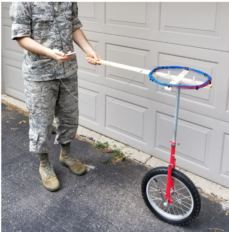
Figure 24: VLF Loop antenna mounted to a unicycle. Note the iPhone 5C is held in order to record locations manually.
