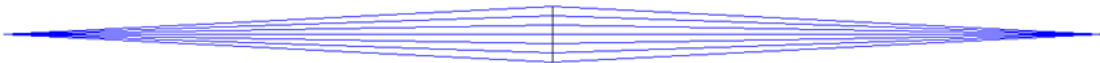
Figure 25. Primary Photon Sieve Ray Fan. A point source placed at a distance 2f to the left of the sieve is imaged at a distance 2f to the right of the sieve. The image will be inverted but unmagnified.
