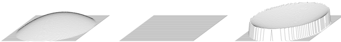
Figure 35. Primary Wavefront Depiction Prediction at Various Wavelengths. The Zemax-predicted wavefront is shown at 736 nm, 740 nm, and 744 nm (left to right) after passing through the primary photon sieve. The outer wavefronts each show approximately 18 waves of aberration and therefore indicate wavelength-specific performance degradation and a limited bandwidth.
