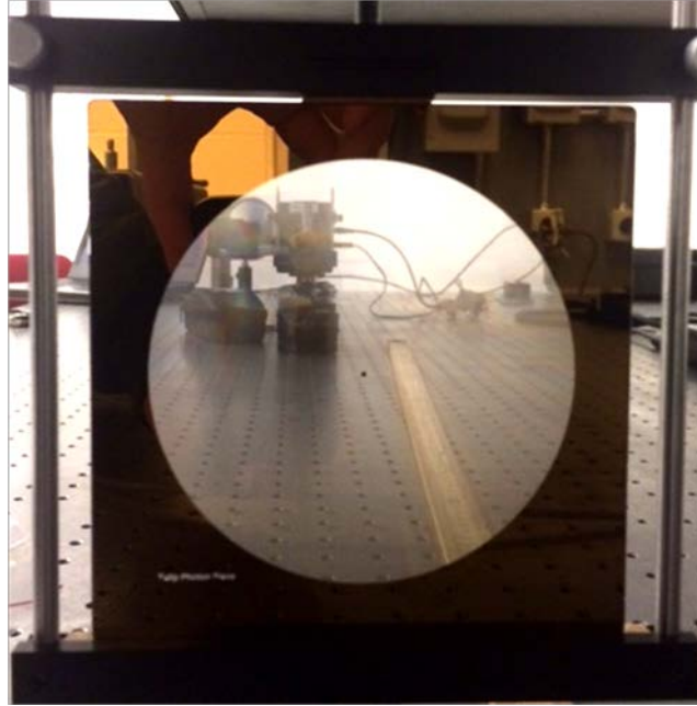
Figure 23. Primary Photon Sieve Image. The sieve was created by printing the hole pattern in chrome on a quartz substrate. It has a 10-cm diameter and a focal length of 0.5 m. There are 3,376 rings and 71,715,741 holes with sizes ranging from 329.04 \mu\text{m} (center) to 5.65 \mu\text{m} (edge).
