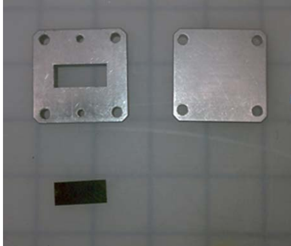
Figure 17. The fixture on the left is the waveguide used for sample mounting for network analyzer measurements. On the right is the shielding block used in calibration, and on the bottom left is a sample.
