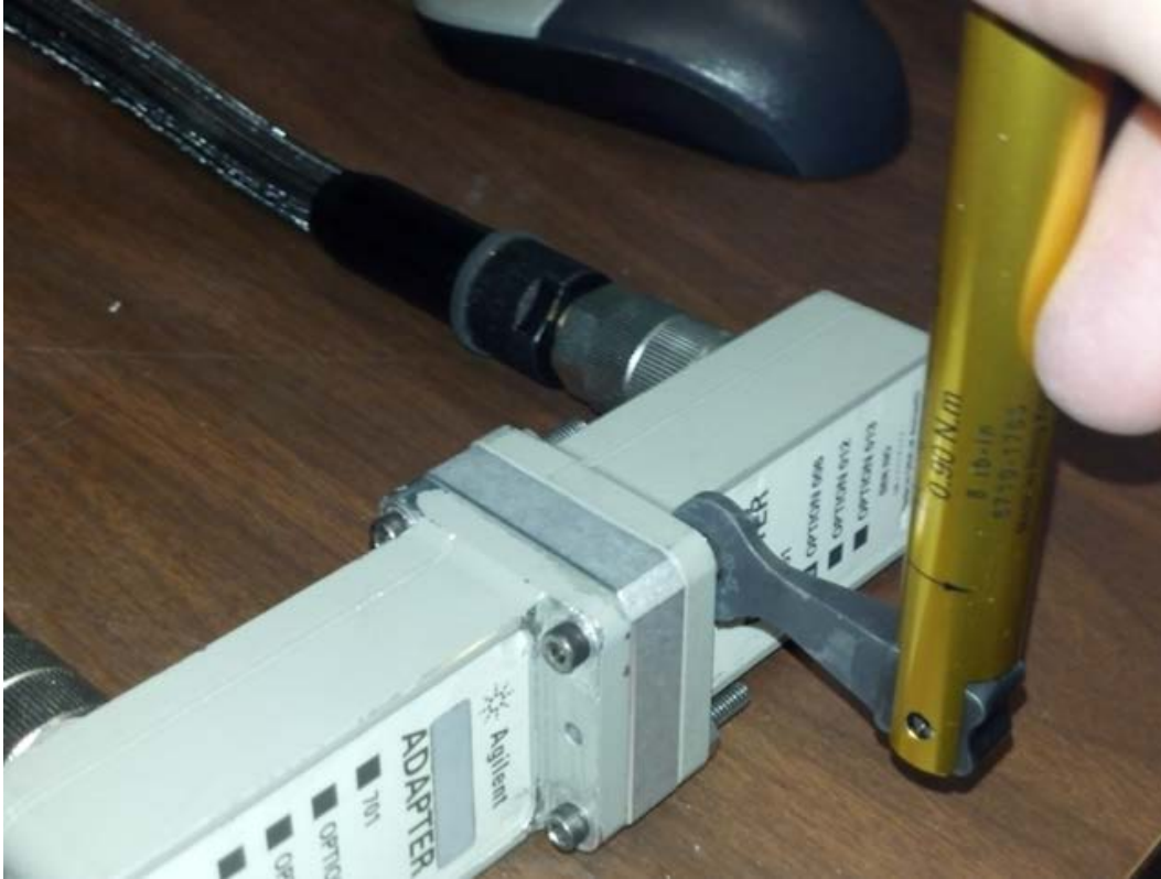
Figure 18. Photograph showing a sample being secured into the Agilent Technologies E8362B PNA Series Microwave Network Analyzer. The waveguide is secured by hex cap screws and nuts tightened to the torque specifications of the Agilent Technologies 0.9 N-m torque wrench. The left side is the port adaptor for port 1, and port 2 is on the right side of the photo.
