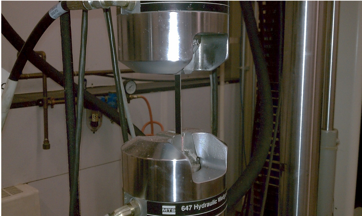
Figure 16. The sample mounted in the MTS 810 ready to begin the monotonic tension test.
