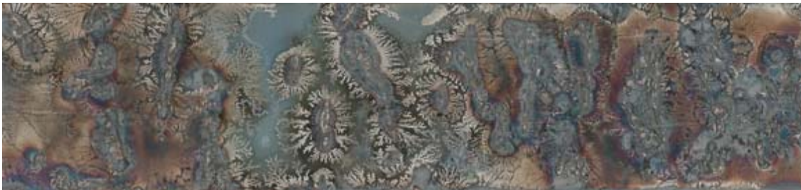
Figure 24 – A developed film destroyed by contact with aluminum.
