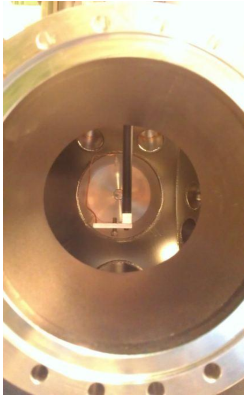
Figure 27: Performing a visual alignment of the sample in relation with the chamber openings and detectors.
