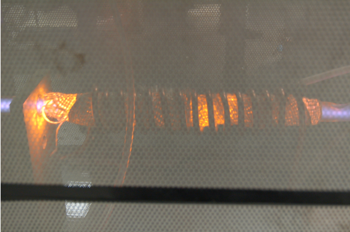
Figure 8. The discharge volume glows brightly along the whole cell but the bright orange Pyrex fluorescence overwhelms the weaker purple glow of the Argon/Helium discharge. A divot in the Pyrex is visible on the right side of the solenoid. This glow became common when working with the IC discharge at pressures above 200 Torr and powers above 800 Watts.
