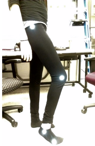
Figure 15. Body Markers. VICON's retroreflective markers are precisely placed on the joints of the lower extremity. Marker #1 is placed on the hip joint near the femoral greater trochanter. Marker #2 is placed at the lateral condyles near the knee joint. Marker #3 is placed near the talocrural ankle joint. Marker #4 is placed laterally near the joint of the fifth metatarsal.
