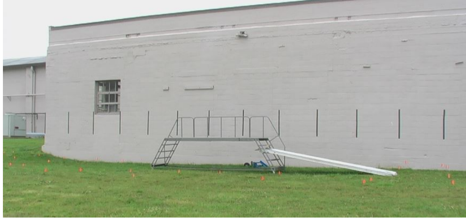
Figure 2. INSPIRE Racetrack. The INSPIRE racetrack included a set of stairs, a crossover platform and a ramp. Exact location of the ramp is 28 feet from the left side of the building, 25 feet from the right side of the building, and 6 feet away from the building. The vertical dark markings, situated every 5 feet, were used for scaling purposes in the video analysis.
