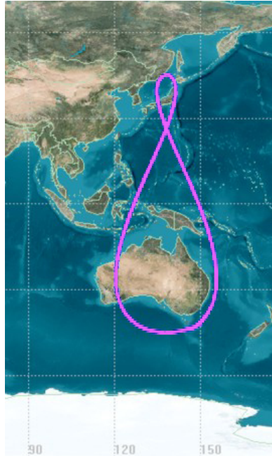
Figure 3.8: Illustration of an analemma pattern traced out by a GEO satellite over the course of one year. This is only a specific example and does not account for all GEO satellites
