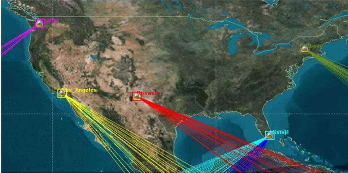
Figure 4.8: Resulting layout of locations needed to use the spherical reflector to communicate with all GEO satellites over the CONUS. Note that the specific latitudes of these locations is of interest and the city names are merely for reference.
