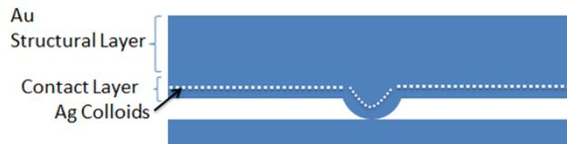
**Figure 22 Example Diagram of Ag-Au Beam**
