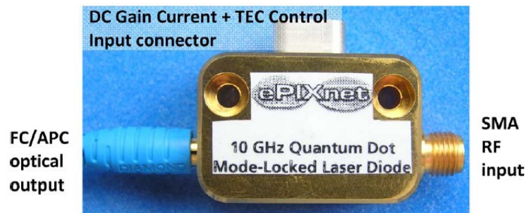
Figure 14: Packaged 10 GHz oscillator [23].
