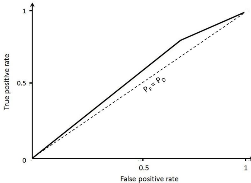
Figure 4.8: ROC curve for the most successful validation result among the Combo validation sets, which results from NASAFS-IDF1 features and a decision tree classifier. The Combo dataset is validated with data collected with a NC fore optic. The set is comprised of 112 samples of “stress” and “non-stress” and six features.
