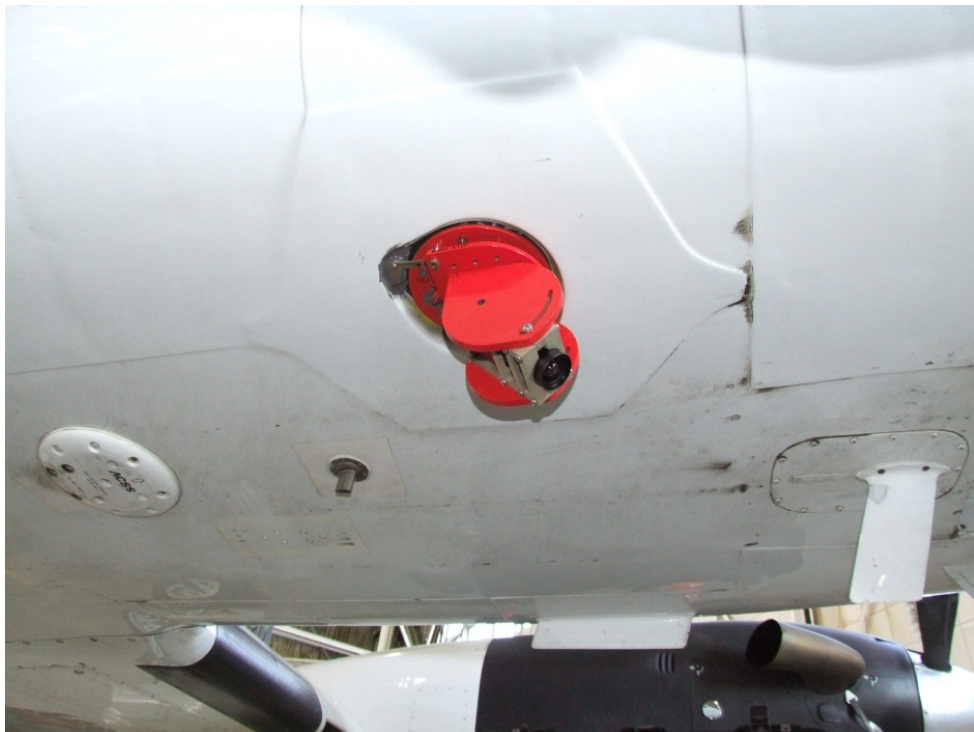
Figure 35. Prosilica camera Installed in the mounting bracket on the underside of the C-12C
