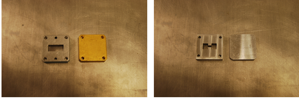
(a) Rectangular Standards: Line (L) and Reflect (R) (b) DRWG Standards: Line (L) and Reflect (R)
