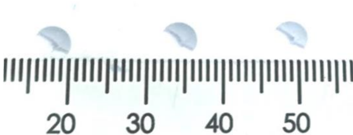
Figure 4.1. Pump beam shape. The diameter of the laser spot was approximately 5 mm, but was concentrated into a crescent shape.
