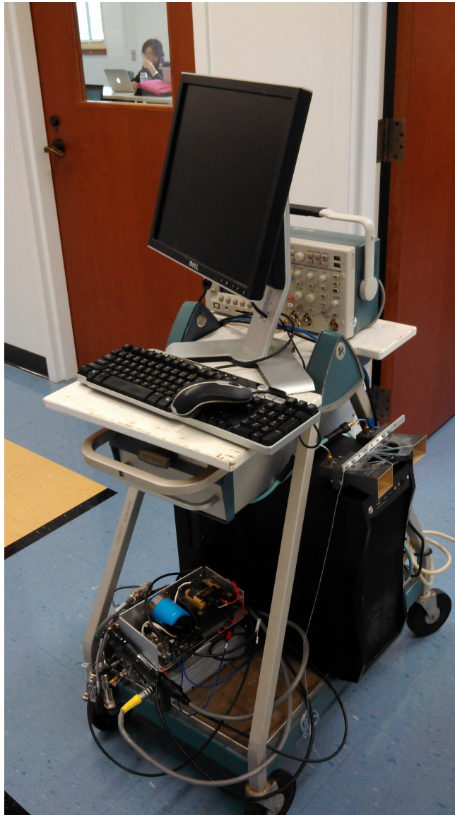
Figure 48: Picture of mobile platform including an ATX computer, INS, UWB-OFDM radar system, and analog front-ends for both sensors.
