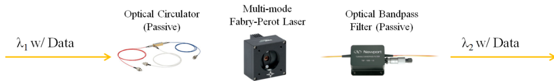
Figure 2: One of the proposed optical-optical methods of wavelength conversion.
