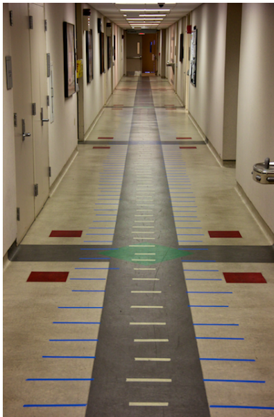
Figure 4.2: The hallway used for both the constant heading and vanishing point transition tests. The pieces of tape were added to the floor to improve the velocity measurements.
