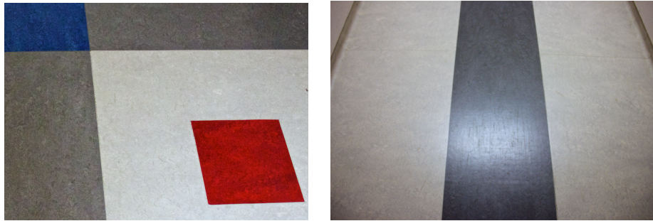
Figure 4.3: Closeup images of the hallway floor. As can be seen the detail in the floor is inconsistent along the course, and does not provide regular enough features for the velocity measurement system.
