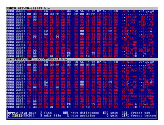
Figure 4.3: VBinDiff of the beginning of FRN20.013 and FRN13.071.
