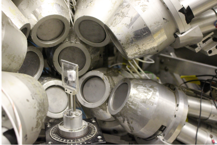
Figure 17. The GEANIE detector array at LANSCE/WNR, with the enriched ^{187}\text{Re} sample mounted in the center of the array. The beam originates from the far right of the array in the photograph. This picture was taken with the detector array opened, so approximately 2/3 of the 18 installed detectors are visible.
