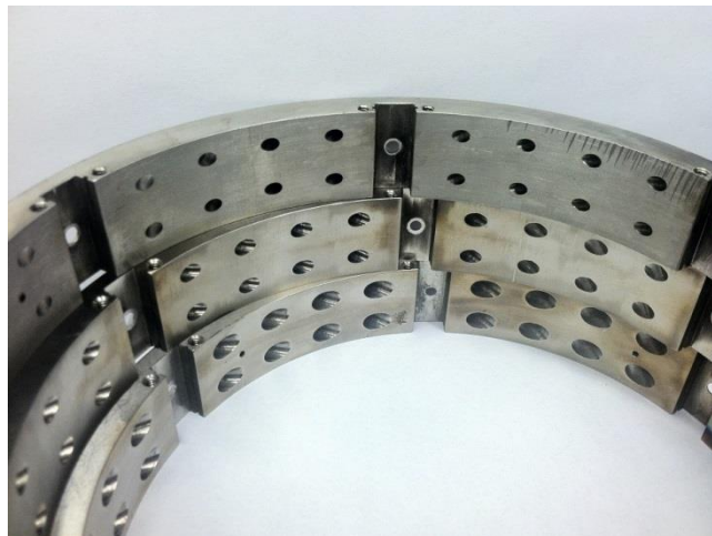
Figure 62. 0.35 cm, 0.45 cm, and 0.65 cm (from top to bottom) diameter air driver rings
