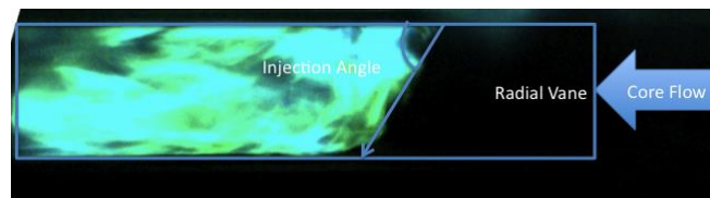
Figure 24. High speed video image of cavity migration angle into the core stream [20]
