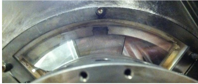
Figure 35. Optical access section at the front of the UCC with overlap from back windows
