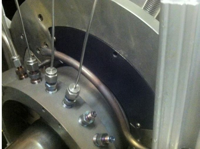
Figure 63. Exit of the UCC with metal inserts in place of the quartz windows on the rear cavity wall.
