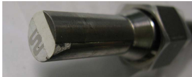
Figure 13. Sensing face of the heat flux gauge
