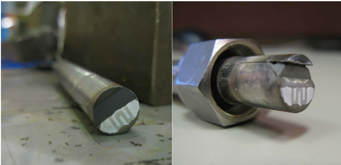
Figure 20. Heat flux gauge before and after data collection
