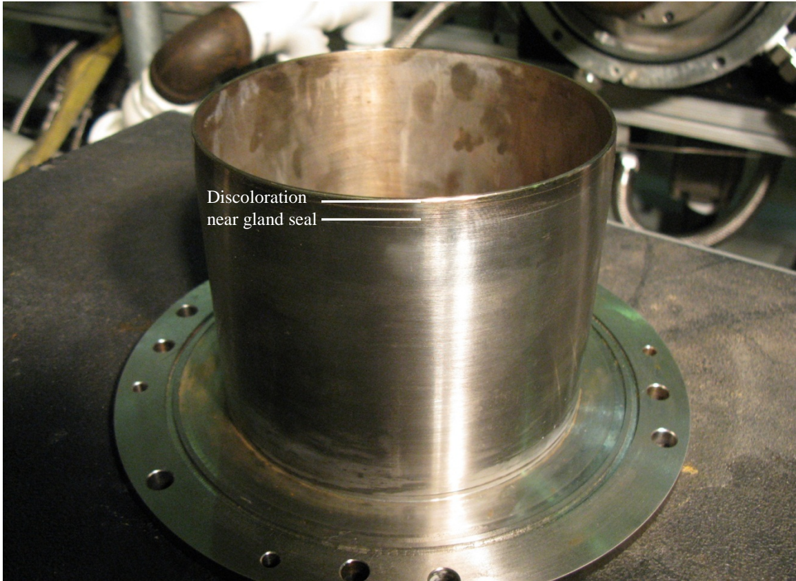
Figure 7. Stainless steel outer body containing wall after two-second operation
