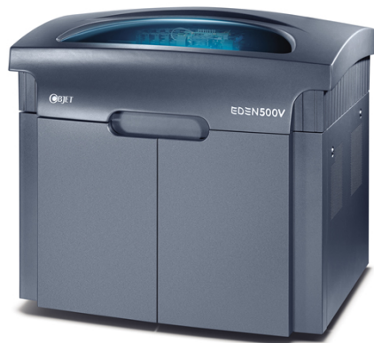
Figure 73: The 3D printer used to fabricate the major parts for the flapping mechanism.
