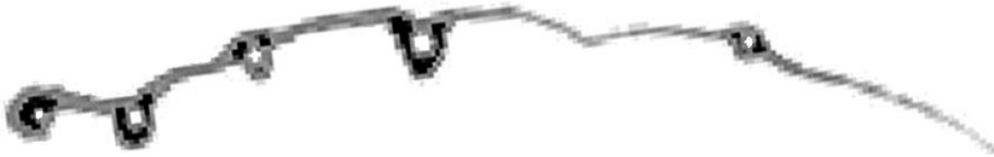
Figure 54: Example of a wing cross section produced through CT scanning. Hundreds or thousands (depending on resolution of the scan) of these images are created as part of the scanning process. These scans are used to determine vein and membrane thicknesses at locations throughout the wing that are used in the FEM.
