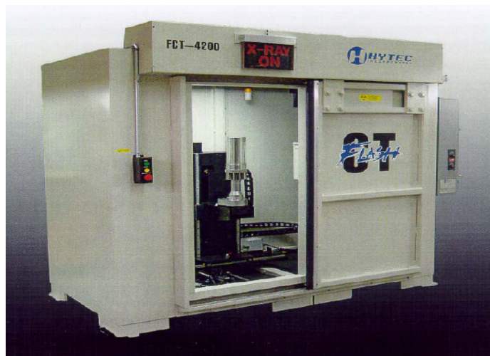
Figure 53: AFRL's computed tomography (CT) machine employed to obtain the three dimensional geometry, with internal vein features of a hawkmoth wing.
