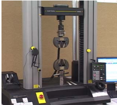
Figure 30: Extensometer machine like the one used to characterize Young's Modulus for the paper beam, clamp validation study.
