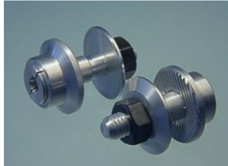
Figure 76: Rear (collet) and front (thread & nut) views of the self-centering, collet-type adaptor used for attaching the drive wheel to electric motor shaft. The collet side of the adaptor attaches directly to the motor shaft. The drive wheel slides over the threaded end and is held in place with the washer and nut.
