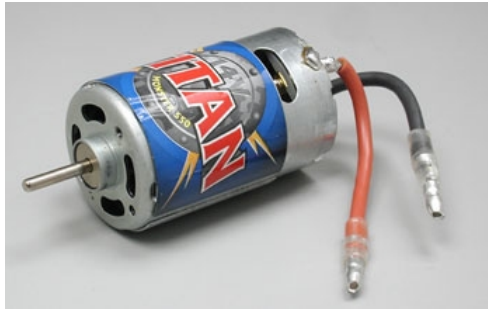
Figure 75: The Titan 550 hobby-class electric car motor used to power the flapping mechanism. Specifications: 14.4V, 23-turn, fan-cooled. Dimensions: 3.07 inches end-to-end; 1.46 inch can diameter; 0.125 inch shaft diameter.
