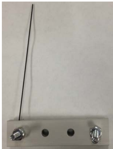
Figure 16. Leading edge beam of the duck wing shown clamped between two plates. The plates were bolted to an electrodynamic shaker for testing.
