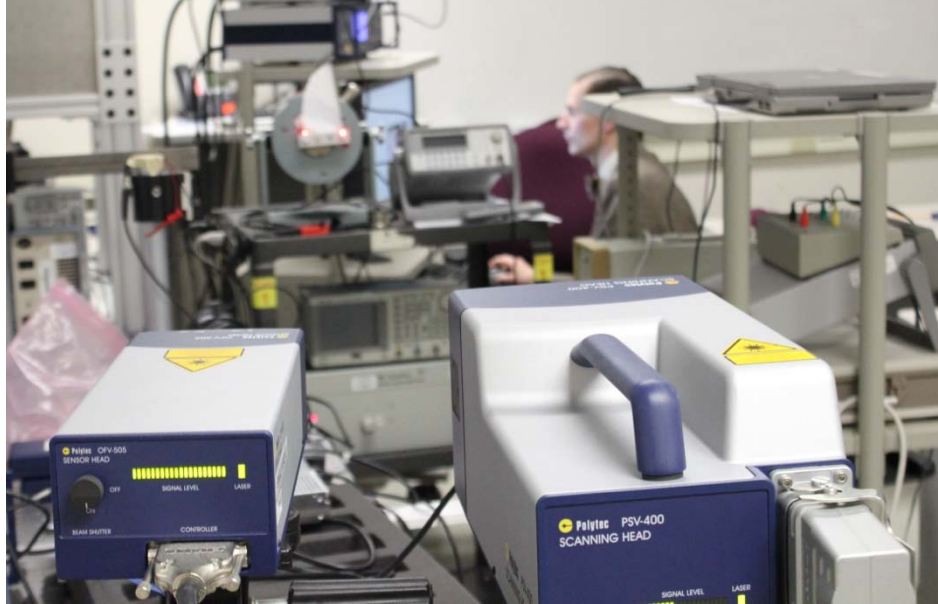
Figure 15. Test setup for the laser vibrometer. The two lasers are located at the bottom of the image with the scanning laser on the right and the reference laser on the left. In the background the wing is shown clamped to the shaker. The same test setup was performed for the leading edge beam.
