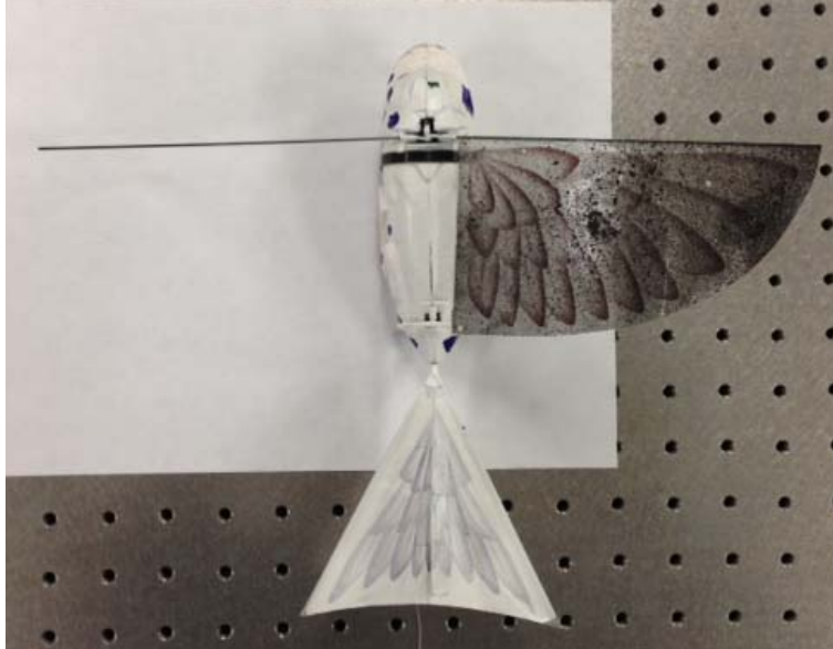
Figure 17. Top view of the test article used for modal testing with the wing membrane removed from the leading edge beam on the left side. This configuration would show different results than the bar in the clamped configuration.
