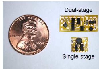
Figure 2.5: Dual and single stage drive circuits for high voltage gains [14].
