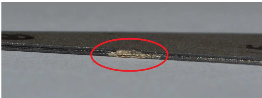
Figure 4.28: Conductive epoxy overflow between layers.
