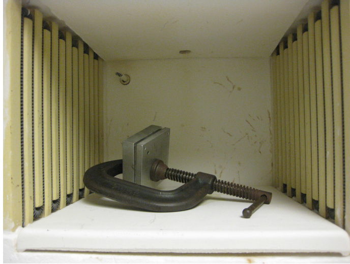
Figure 3.6: Clamp and actuator assembly in oven.
