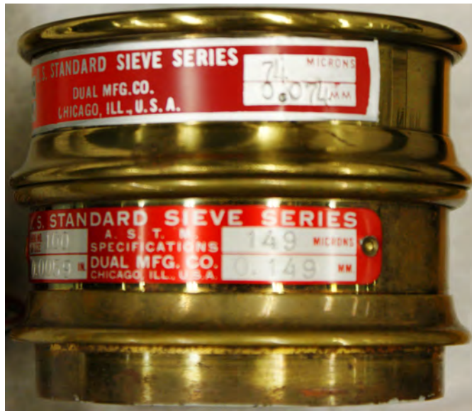
Figure 4.22: Standard sieves used for brushing black laser printer toner powder through for uniform stochastic speckle patterns
