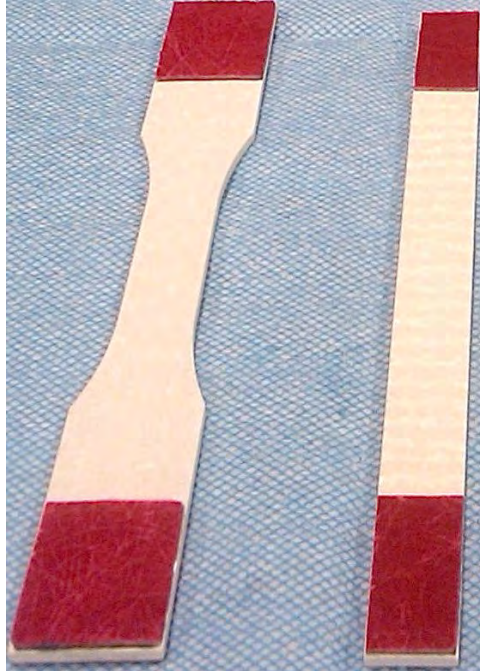
Figure 3.3: Nextel™ 720/AS dogbone (left) and straightsided (right) specimens
