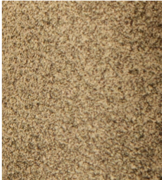
Figure 4.3: Example stochastic, or random, speckle pattern for use with DIC
