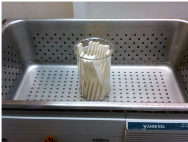
Figure 6.12: DNS specimens during 25 minute ultrasonic acetone bath
