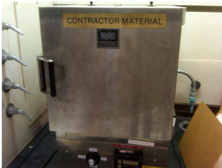
Figure 6.15: DNS specimen bakeout furnace
