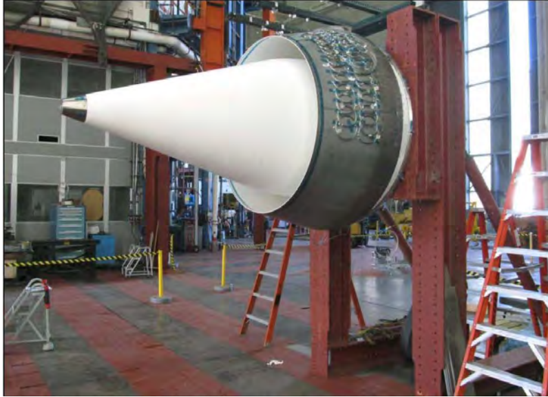
Figure 2.5: CMC turbine engine exhaust nozzle and centerbody (Courtesy Boeing)
