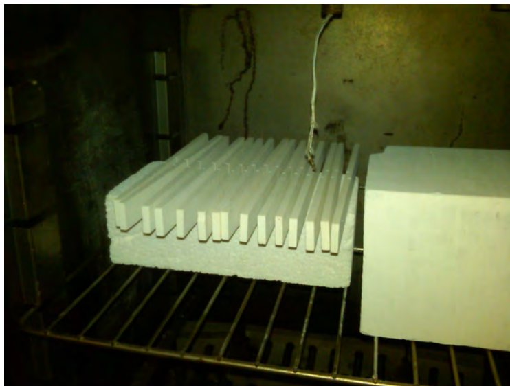
Figure 6.16: DNS specimens bakeout setup
