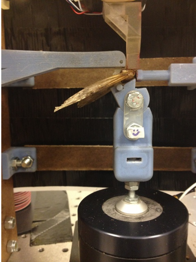
Figure 32: Close-up view of the test apparatus with the specimen in place
