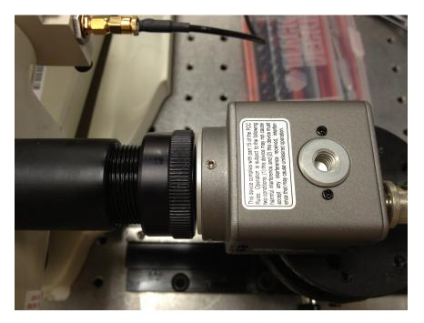
Figure 4.11. The Davidson Optronics D-275 autocollimator (left) operation utilizing a CCD camera (right) to view results through the eyepiece.
