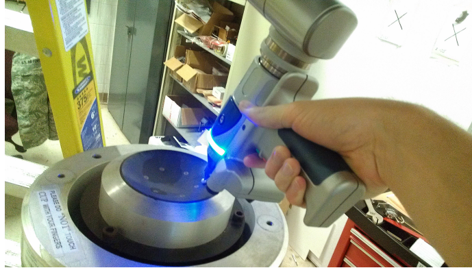
(a) Creating Sphere from Air Bearing to Find Center of Rotation for SimSat
