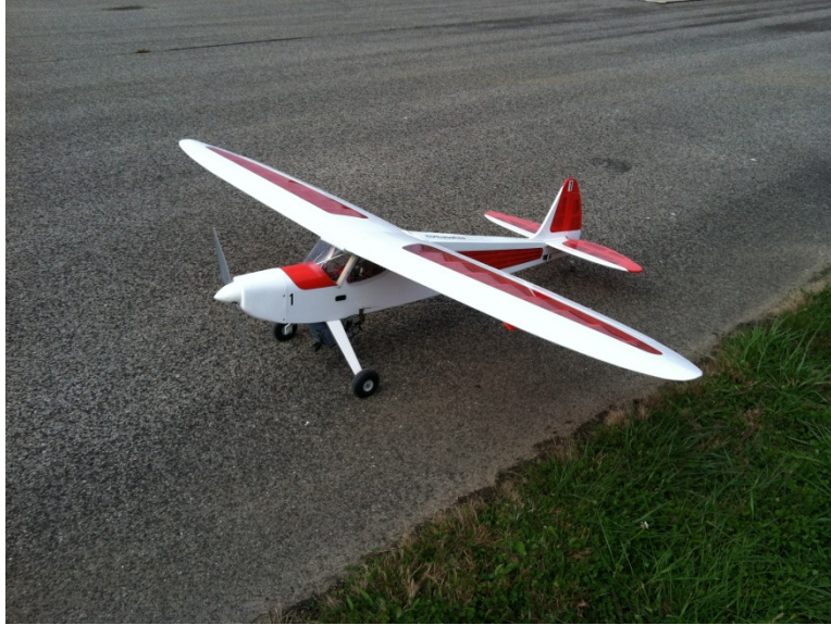
Figure 40: Sig Rascal 110 in flying configuration with MSI sensor payload
