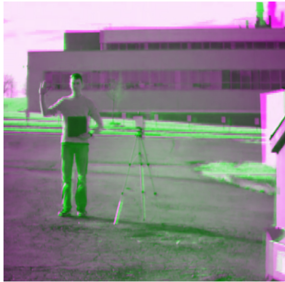
Figure 28: Results of projective transform registration using SIFT and RANSAC. Shows the stereo disparity of the two cameras. RGB is red image, and SWIR is represented by green image. Note that disparity is only minimal at one location, the dismount, whereas disparity increases with greater distance.
