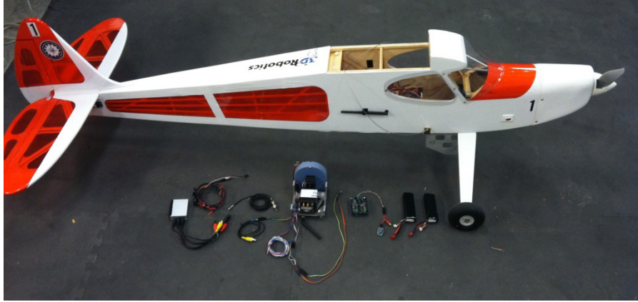
Figure 26: Test Sig Rascal 110 airframe and sensor payload
