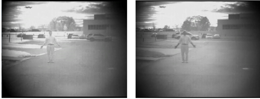
Figure 32: Left, 1050nm image, Right, 1550nm image. Focus is at a mean setting. Note the car in background between the filter change (Filtering speed was 0.50 seconds/filter change).
