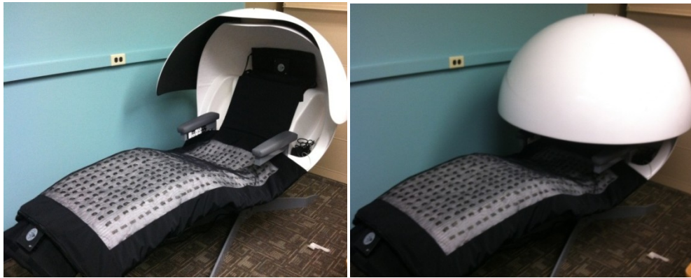
Figure 1. The thermoelectric pad and blanket situated inside the pod while the shield is open and closed.
