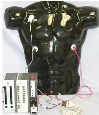
Figure A 3. BIOPAC ® hardware system showing placement of ECG electrodes.
