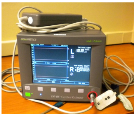
Figure A 2. Somanetics Invos Cerebral Oximeter 5100B (left) and participant wearing adjustable headband and EOG electrodes (right).
