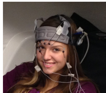
Figure A 2. Somanetics Invos Cerebral Oximeter 5100B (left) and participant wearing adjustable headband and EOG electrodes (right).
