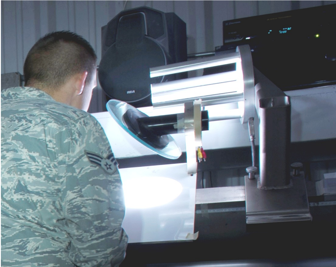
Figure 26. A technician stands in front of the drawing board on the Holloman SOON telescope. White light is reflected down the length of the telescope to the 45° mirror. This image is then reflected down on the drawing board where solar analysts record all the sunspots visible on the AFWA form 21 from Figure 25. The guide instrument is visible above the 45° mirror while the rail along which the drawing board can slide can be seen with a measuring tape running its length.
