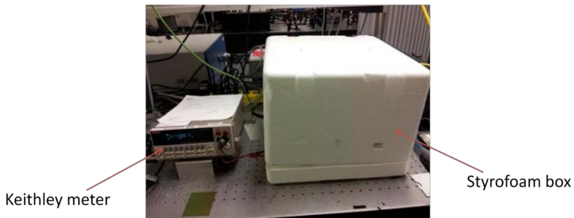
Figure 16: Laser pigtail source, lens and sample holders are enclosed in a Styrofoam box for better insulation. Small holes are made to the side of the box to attach connectors from the Keithley meter to the thermocouple wires.
