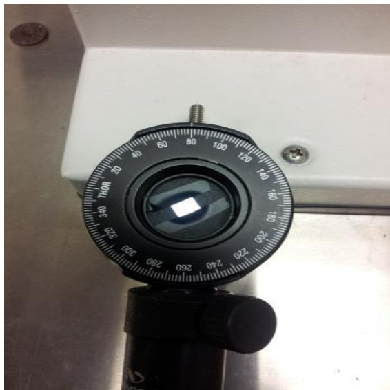
Figure 29: Sample mounted to the dial (Part 2 from Figure 28). Transmission measurements were taken as the dial was gently rotated by five degree increments.
