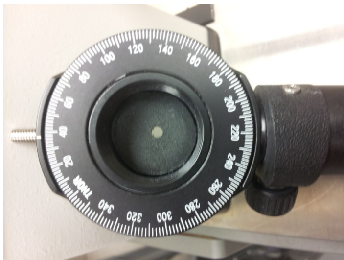
Figure 58: The sample holder hole was misaligned with the center of the FTIR beam. This caused clipping of the incident beam and non-uniform transmission through the sample holder to the detector.
