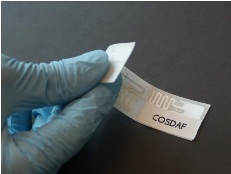
Figure 2.13: A printed RFID tag on flexible substrate [35].
