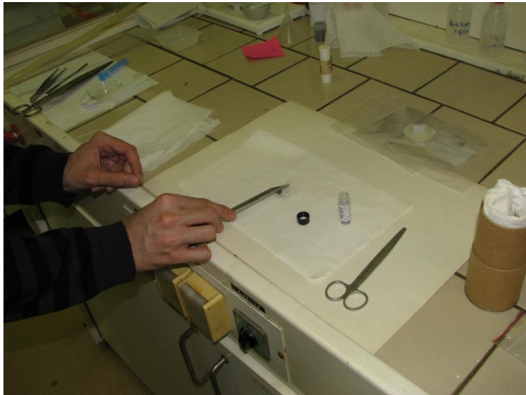
Figure 12. Preparation of the enriched ^{185}\text{Re} metal powder target. The target was contained in a small Teflon bag and adjusted such that homogeneity was maximized without having to incorporate a solvent.
