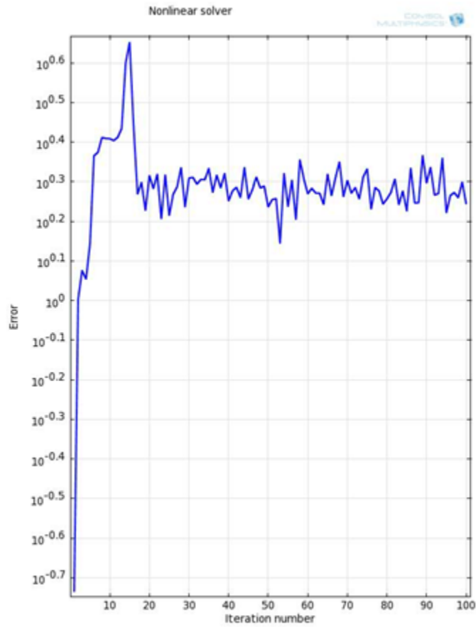
Figure 37. Note that the error associated with solving the model remains high and, indeed, gives no indication that it would converge for any number of iterations.
