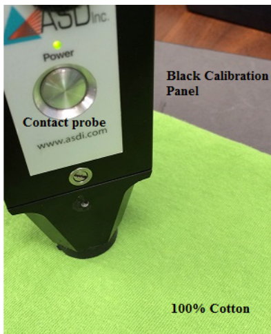
Figure 3.1: Laboratory setup of reflectance data collection. The green, 100% cotton shirt sample, contact probe, and black calibration panel used are labeled.
