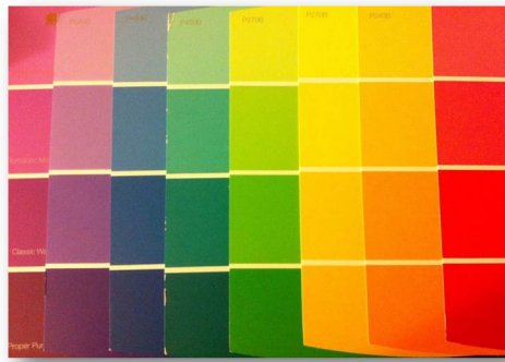
Figure 3.3: Color chip samples used in feature selection for visible spectrum. From left to right, the color schemes are: purple, indigo, blue, turquoise, green, yellow, orange, and red. Each color scheme has four shadings, separated by horizontal white lines.
