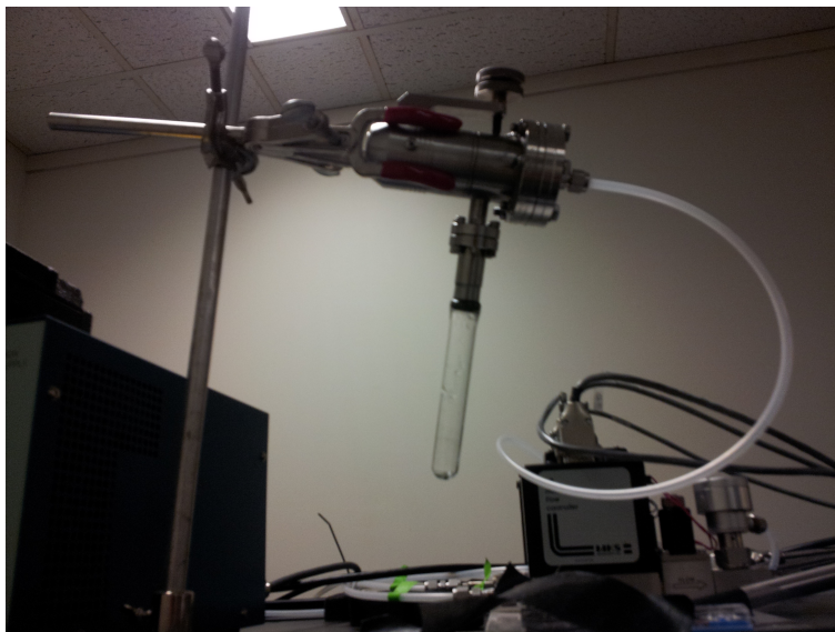
Figure 3.6: The water vapor concentration inside the growth chamber is controlled using a test tube containing water with a leak valve. The leak valve is not computer controlled but the water concentration is measured using a Shaw Superdew 3 dew point meter. [38]
