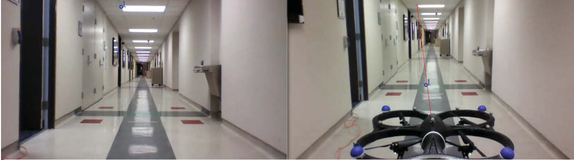
Figure 4.6: An Erroneous Match With Good Parallax Angle. This figure shows a possible scenario in which the intensity of a light fixture is erroneously matched to reflections on a floor tile. The image coordinates of the light fixture in the left image map to a line which passes through the true feature location and converges at the epipole in the second image.
