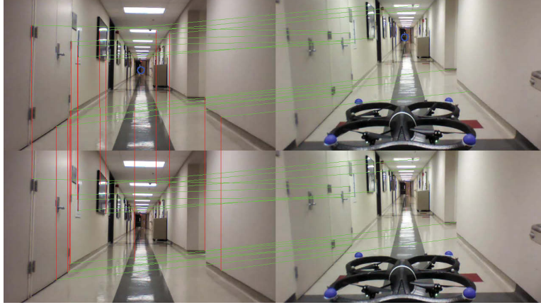
Figure 3.4: Results of Feature Correspondence. The image is a stitching of the images of the leading (left) and trailing (right) vehicles at the current time (top) and the previous time (bottom) epochs. Green lines indicate a match across cameras. Red lines indicate a match across time epochs.
