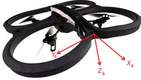
Figure 2.5: Body Frame of the ARDrone. In this frame, the x -axis extends out from the nose of the vehicle, the y -axis extends out the right wing, and the z -axis extends downward [18].
