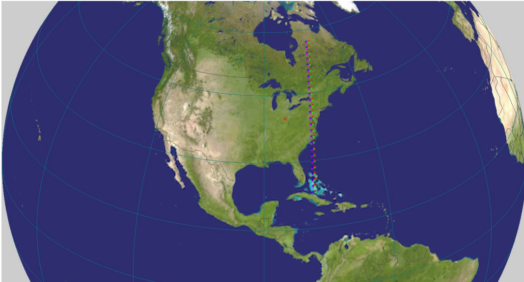
Figure 3.3: The portion of the orbit considered in this research does not pass directly over the target. The red star represents the target and the colored asterisks represent the Cubesat positions over time.
