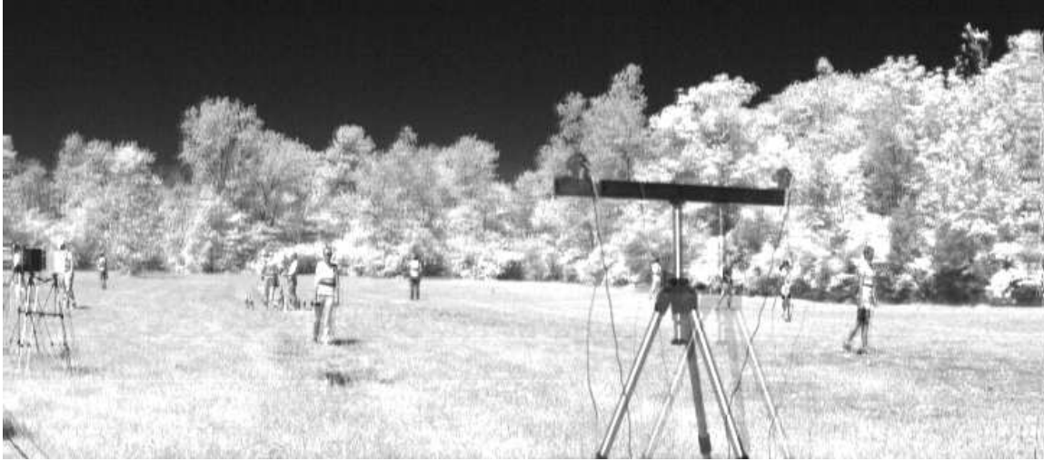
Figure 4.4: A layer in the HSI image at wave band 1007 nm. As can be seen in the figure, the ghosting effect indicates the transition from the AisaEAGLE to the AisaHAWK. This requires image registration to correctly align the two sensors.
