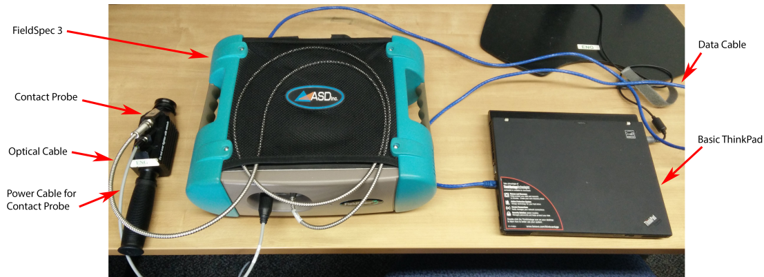
Figure 3.1: FieldSpec ® 3 with contact probe and ThinkPad. The contact probe is connected to the FieldSpec ® with the optical cable and the power cable. The power cable power the built in illumination source and the optical cable collect and transmit the electromagnetic energy to the FieldSpec ® 3. The FieldSpec ® 3 is used to process, analyze, and interpolate the data. The data cable transmits the processed data from the FieldSpec to the RS 3 software in the ThinkPad.
