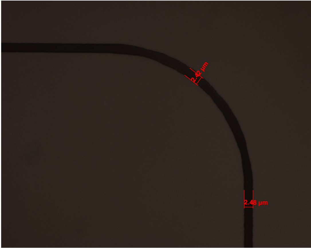
Figure 29. Filleted corner of cantilever is used to reduce stress in the membrane caused at the sharp right angle that previously existed. The tight \sim 3 \mu\text{m} gap is still maintained throughout the corner.
