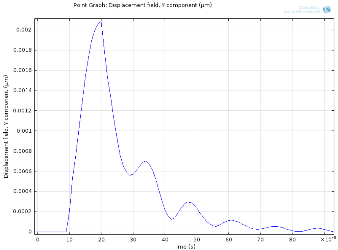
Figure 13. 5 \mu\text{m} thick bimetal cantilever tip displacement
