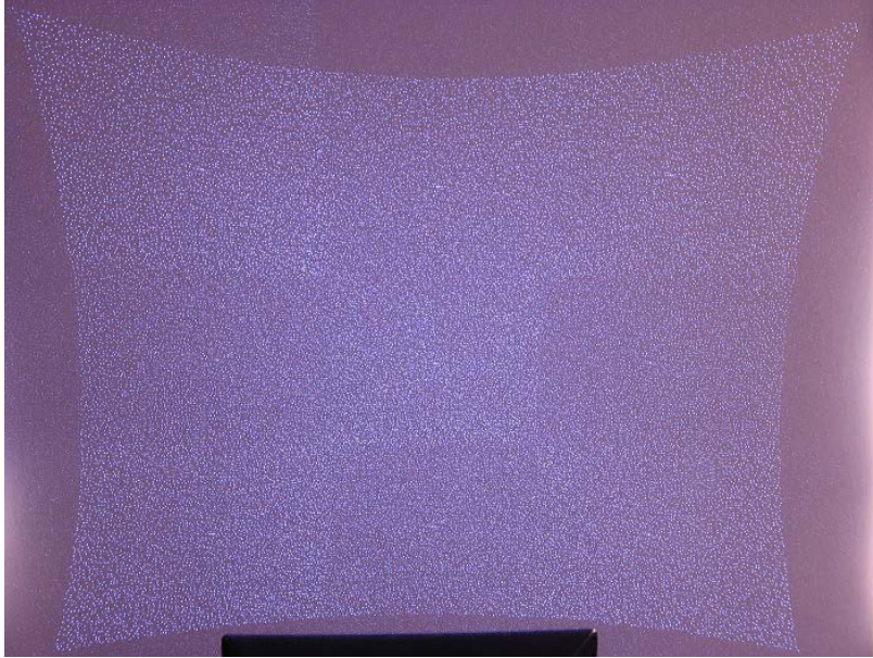
Figure 2.4: Kinect Speckle Pattern. This pattern is projected by the IR emitter of the Kinect. The reflected pattern is then received by the IR receiver, and compared to the known reference pattern that was projected. Based on the differences between the reflected pattern and the reference pattern, calculations are performed to determine the depth of objects within the scene. Sourced from the FuturePicture series on Kinect Hacking [22].
