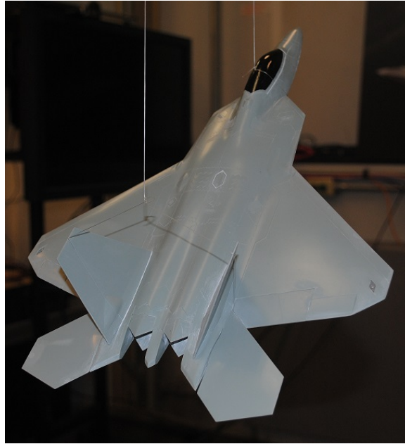
Figure 3.3: Suspended Subject Airplane Model. The 1/48th scale F-22 model is suspended from the ceiling using fishing line, directly over the center of the turn table in Figure 3.1. For the experiment, the aircraft was kept at an approximate 43^\circ nose up, or pitch, angle. This was necessary for the sensor to be able to see both the top and bottom surfaces of the model in a single rotation.
