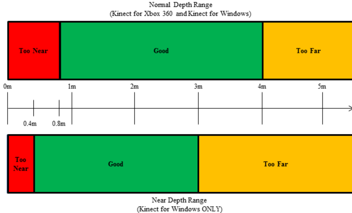
Figure 2.5: Kinect Depth Ranges. This diagram depicts the differences in the two range modes available in the Kinect for Windows variant of the sensor. Note that the Kinect for Windows can operate in either the normal or near range, and the original Kinect for Xbox 360 can only operate in the normal range.
