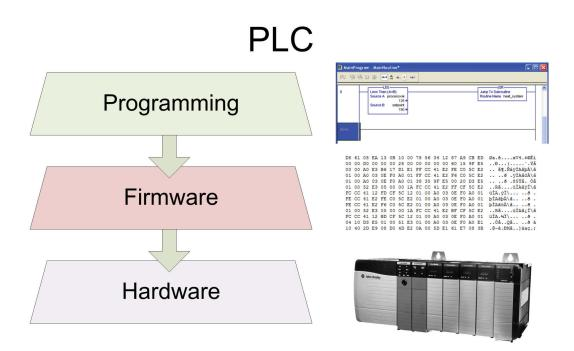
Figure 2.2: PLC Composition Layers [49]
