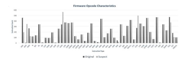
Figure 3.2: Histogram Displaying Contrasting Opcode Counts for Two Firmware Files
