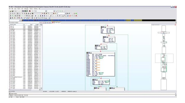
Figure 2.10: IDA Pro Program Displaying a Disassembled L61 Firmware Function [25]
