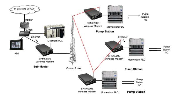
Figure 2.1: Pump Station to Sub-Master PLC Network [58]
