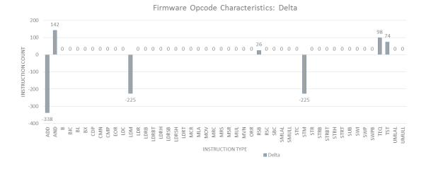
Figure 3.3: Histogram of the Difference Between Base and Suspect Histogram Counts
