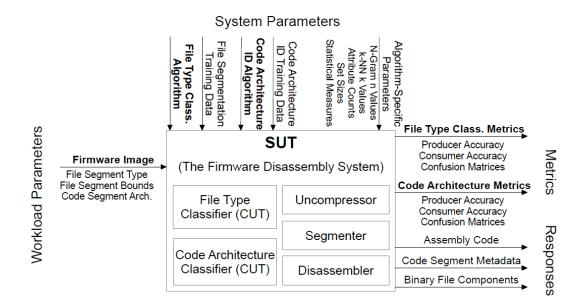
Figure 2.6: Sickendick's Firmware Disassembly System [64]
