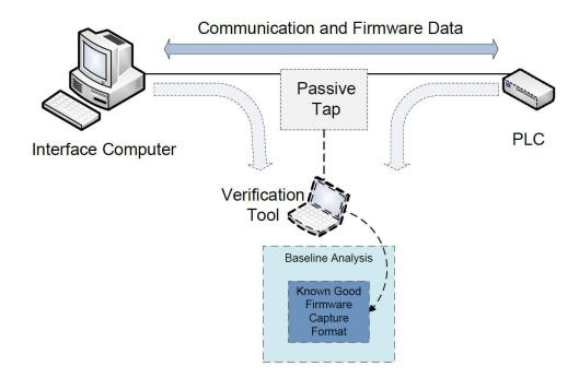
Figure 2.4: McMinn's Passive Capture and Baseline Analysis Experiment [50]
