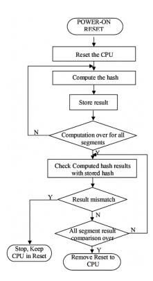
Figure 2.3: Khan's FPGA/PLC Control Flow [30]
