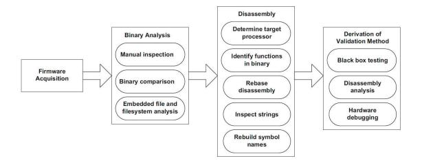
Figure 2.5: Basnight's Firmware Reverse Engineering Process [3]
