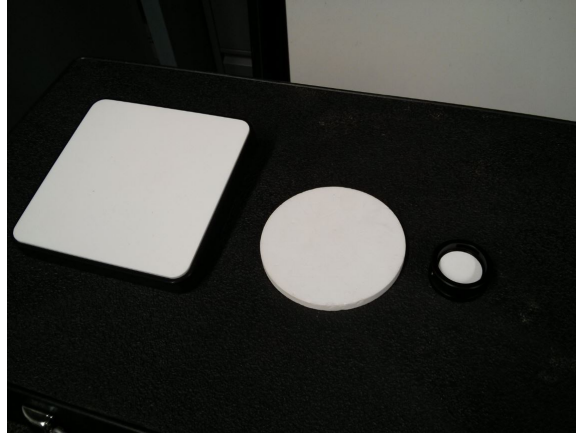
Figure 3.3: An image of the three white reference panels used in the experiments.
